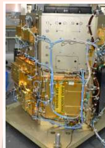
Integrated P band ASAR Payload
