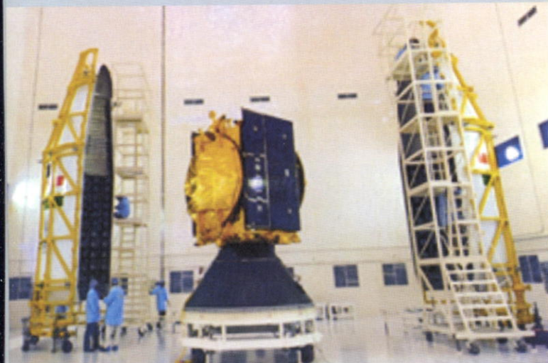
Two halves of GSLV-D5 payload fairing surrounding GSAT-14 satellite
